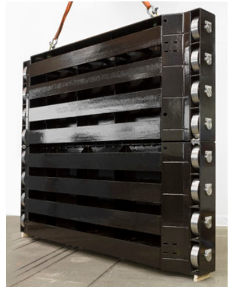
Penstock gate-roller gate, KW Moorburg, W x H = 4,800 x 3,900 mm for 2.8 bar made of steel – coated 4 times
